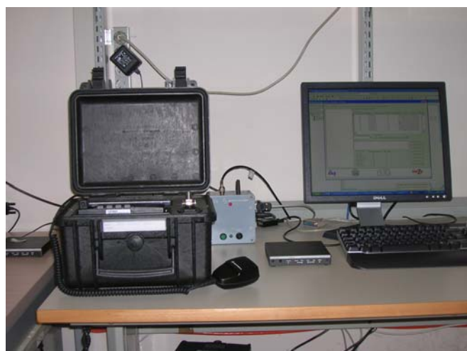
Figure 3 Prototype Local Element: VHF radio station, Nav/Com module and PC.
