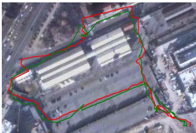
Figure 9 Dynamic test in urban environment. User Terminal based positioning (red trace) vs. network-based positioning (green trace)
