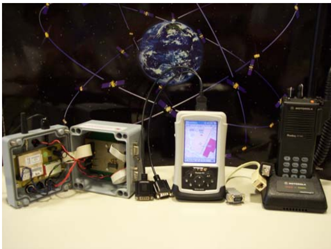
Figure 4 User Terminal equipment: the prototype navigation and communication unit, the PDA and the VHF radio transceiver
